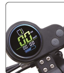
Speed control throttle/ on-off button/battery indicator
