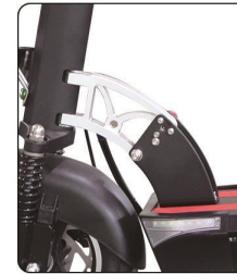
Quick folding mechanism self locking/release grip
